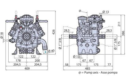
$\Delta$  In C/SP pumps the value  $\Delta$  17 is reduced to 15 with the seal ring flange mounted on the pump body. N.B. Remove the seal ring flange code 1400140 before fitting the reduction gear to the pump.
