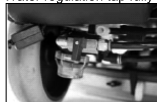
Fig. 9 Water regulation tap fully closed
